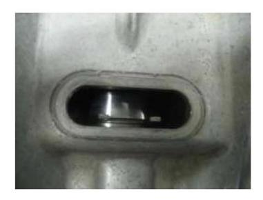
Reinstall the speed sensor and rubber plug. Use a bit of the silicone sealer to seal the threads on the sensor as well as around the rubber seal for a tight, leak proof seal.
