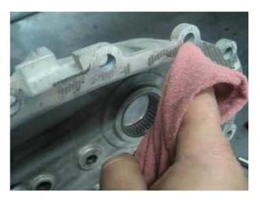
Use the supplied silicone sealer with the dispensing nozzle and apply a 3/16" wide bead of silicone sealer around perimeter of case on center of flange. It is not necessary to go around the bolt holes. Apply the sealer in board of the bolt holes as shown.
