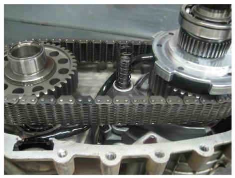
Locate the dowel pins and place them in the front half of the transfer case. They may be in place or they may have come out with the rear half during disassemble. There is one dowel pin on each side, identified by a counter bore in the case. Both of these must be in place or severe damage to transfer case could occur.
