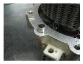
Cleaning the old silicone sealer off the case is actually pretty easy. Use a rag and simply scrub it off as shown in the picture. You will notice that the flange has a rough finish, this is intentional to promote a good bond with the sealer between the halves. Thoroughly clean the flanges with brake clean or similar to remove all oil. Silicone will not seal properly when oil is present. Failure to ensure area is clean could result in a leak.
