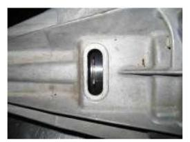
Then use a ¾" wrench to remove the speed sensor. You can see the reluctor wheel inside the case.
