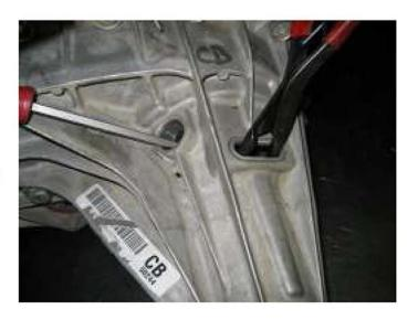
Make sure that the snap ring is locked into place in the bearing and in the housing.
