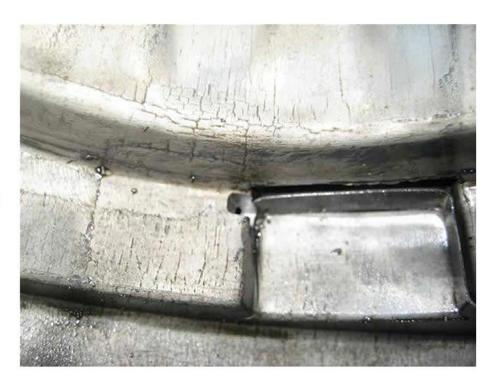
The highlighted box shows what you would expect to see when looking from the outside. Also notice the grime buildup from the fluid leaking and catching road debris. This hole is pretty obvious, but you may start noticing oily buildup towards the back.
