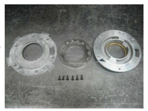
Place the pump upgrade with the tabs up and place the gears back in. After installing the gears, put a few drops of oil on the gears to help with initial lubrication.
