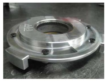
Reassemble the transfer case by reinstalling the pump, reluctor gear and support bearing followed by the snap ring. Reinstall the pickup tube into the pump making sure that the o-ring is in tact.
