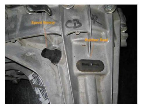
Start by using a screwdriver to pry the plug out of the case. You will see a snap ring under the plug as shown far right
