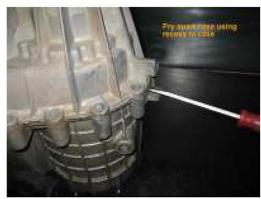
Separate the rear housing be pulling it away from the rest of the case. I find it easier to work on by propping the unit in an upright position as shown.
