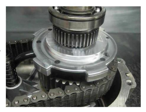
Here is what you should see after reassembly. Make sure that the spring is in place on the shift shaft as well.
