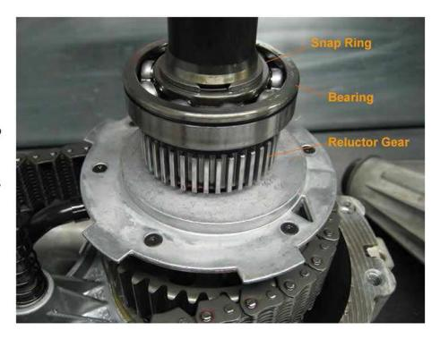
After the bearing is removed, slide the reluctor wheel up and off, notice the orientation of the reluctor. There is a stepped edge that must be reinstalled towards the pump.
