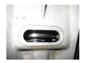
Pry the case halves apart with a flat blade screwdriver at the spots shown.
