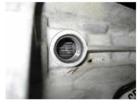
Using snap ring pliers and a straight blade screwdriver, open the snap ring then gently pry on the reluctor gear pushing it forward. This releases the rear support bearing from the rear housing
