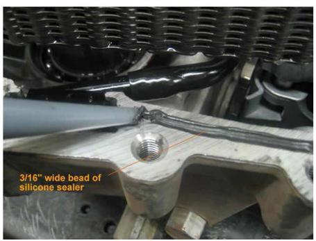
Reinstall the rear housing and install and tighten the housing bolts. Torque to 27 ft lbs in a diagonal pattern. Don't forget to reinstall the brackets as shown.
