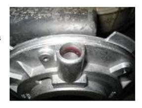
Using a T-15 Torx bit, remove the 6 screws holding the pump together. Here is a disassembled view of the pump. Clean and dry all parts. The pump body may be discarded, it will not be reused.
