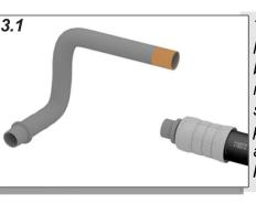
The cut ends of the steel line need to be deburred before installing the repair kit. A piece of scotch bright or emery paper works well for this, as well as removing any light surface debris.
